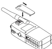
the belt clip down onto the plastic tab.
